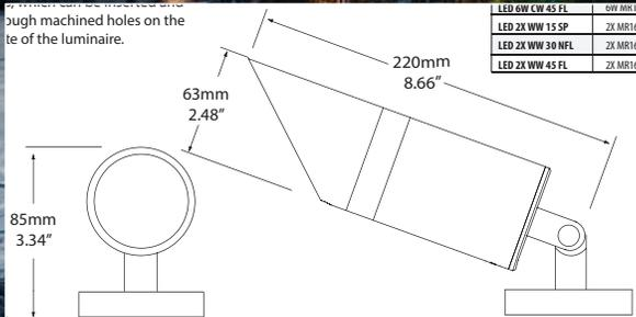
Artemis, Illumicare's adjustable wall mount directional luminaire, is a precision engineered fixture designed for spot, up, and down lighting applications where you need the fixture to be elegant, yet unobtrusive. The contemporary design of the shroud masks the lens and directs the light output to eliminate unsightly glare.
